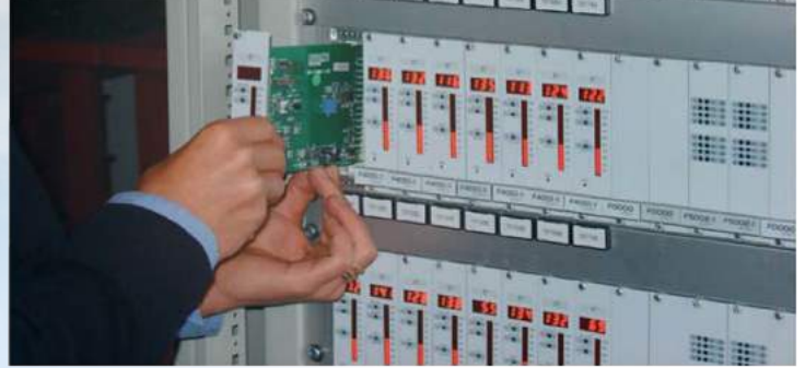
Hot swap of cards, with consequent no need for panel shutoff
