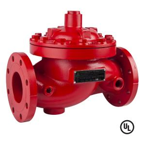
position, water pressure is transmitted through an external bypass check valve and restriction orifice from the system supply side to the top chamber, so that supply pressure in the top chamber act across the diaphragm operated clapper which holds the seat against the inlet supply pressure because of the differential pressure design.
