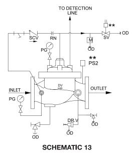
SCHEMATIC FOR DRY PILOT BASIC TRIM WITH DRIP AND DRAIN TRIM FOR HORIZONTAL MOUNTING
