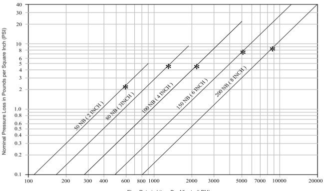
(\* Flow at 15 feet per second [4.57 meter per second])
