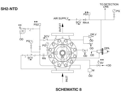
Deluge Valve Swing Check Valve DV Valve  $\triangleright \lhd$  $\mathbb{N}$ Solenoid Valve Angle Valve SV By User ---\*\* Dry Pilot Actuator Sprinkler Alarm (WMG) Optional DPA G  $\vdash$ Restriction Nozzle (Air Line) **Emergency Release Station** Strainer RN-A Μ SCV Swing Check Valve RN Restriction Nozzle (Priming Line) OD Open Drain PS1 Low Air Alarm Pressure Switch PG Pressure Guage PS2 Waterflow Pressure Alarm Switch
