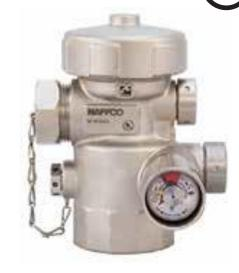
The burst disk allows actuation of manual and pneumatic release devices. When this disk bursts by means of the release system connected to it, the valve opens. Its set pressure does not allow bursting caused by cylinder over pressure.
