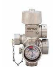
The burst disk allows actuation of manual and pneumatic release devices. When this disk bursts by means of the release system connected to it, the valve opens. Its set pressure does not allow bursting caused by cylinder over pressure.
