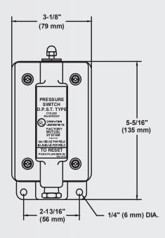
The pressure switch is a double pole, single throw switch housed in a weather-proof back box. After the activation of system, the CO2 pressure from discharge piping operates the switch.
